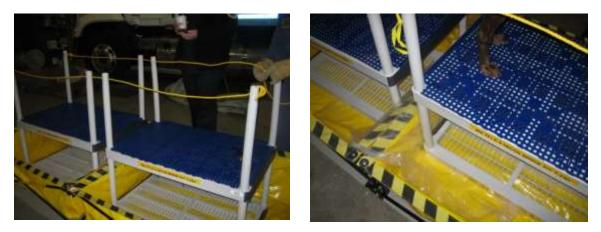
Assembled shelving units are placed within the two pools: one for the initial soap decontamination, next for water rinsing. A plastic sheet has been placed between the two pools to prevent contaminated water from falling through.
