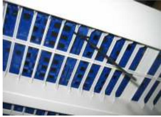
Cable ties are used to secure the flooring to the shelf. This is to prevent the floor from slipping during the decontamination procedure.
